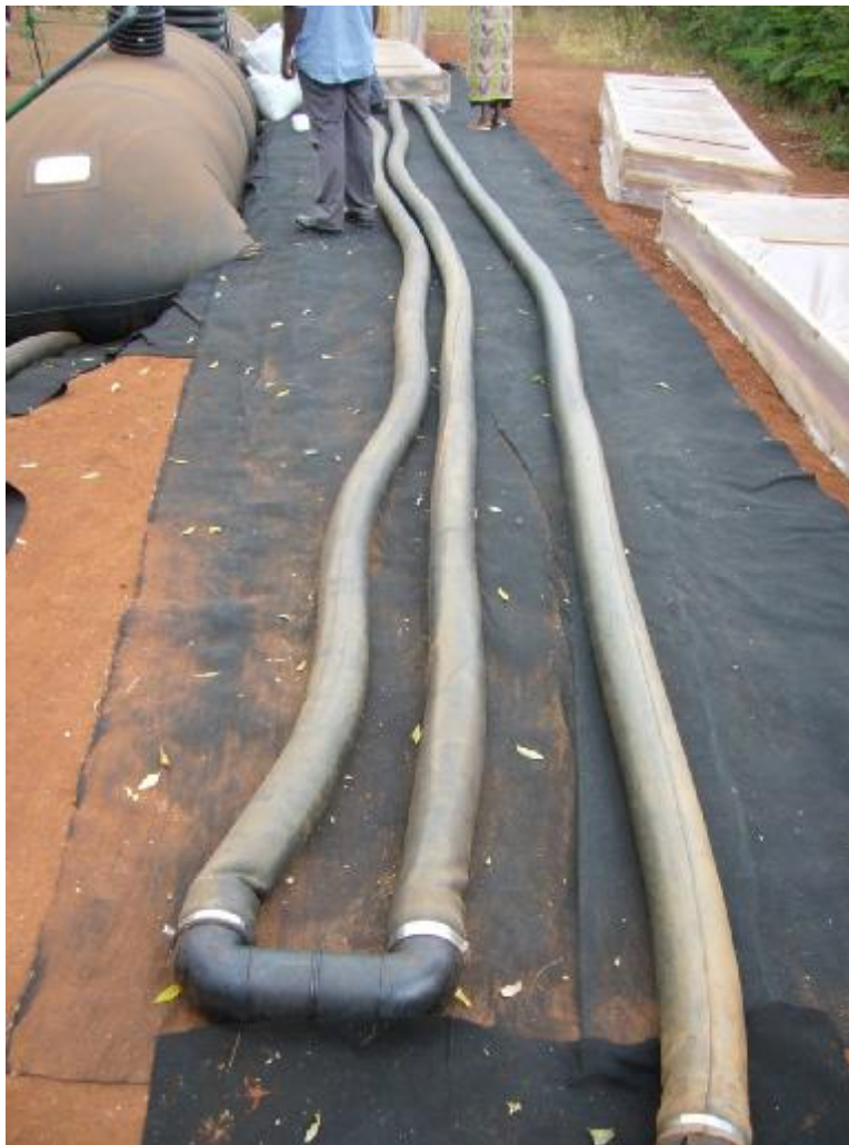
Flexigester trials June 2014, temperature will be increased by plastic 'greenhouses' on top of the effluent pipes (white boxes)
