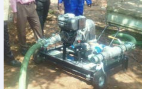
Fig 3: Diaphragm sludge pump.
