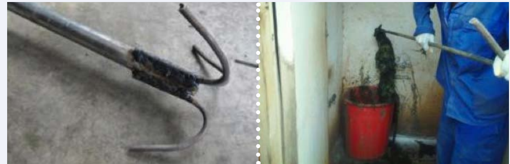
Figure 3: a) Fishing tool. b) Fishing out rubbish.
