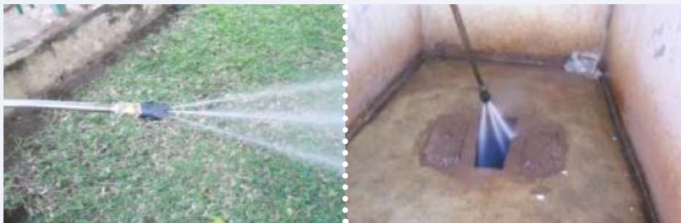
Figure 2. Spray pattern fluidizer using a 4 jet nozzle at 100 bar.
